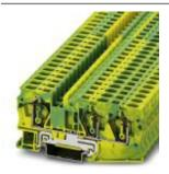
Ground modular terminal block, connection method: Spring-cage connection, number of connections: 3, cross section: 0.2 mm² - 10 mm², AWG: 24 - 8, width: 8.2 mm, color: green-yellow, mounting type: NS 35/7,5, NS 35/15
