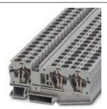
Feed-through terminal block, nom. voltage: 1000 V, nominal current: 41 A, connection method: Spring-cage connection, number of connections: 3, cross section: 0.2 mm² - 10 mm², AWG: 24 - 8, width: 8.2 mm, color: gray, mounting type: NS 35/7,5, NS 35/15
