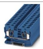
Feed-through terminal block, nom. voltage: 1000 V, nominal current: 57 A, connection method: Spring-cage connection, number of connections: 2, cross section: 0.2 mm² - 16 mm², AWG: 24 - 6, width: 10.2 mm, color: blue, mounting type: NS 35/7,5, NS 35/15
