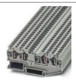
Feed-through terminal block, nom. voltage: 800 V, nominal current: 32 A, connection method: Spring-cage connection, number of connections: 4, cross section: 0.08 mm² - 6 mm², AWG: 28 - 10, width: 6.2 mm, color: gray, mounting type: NS 35/7,5, NS 35/15
