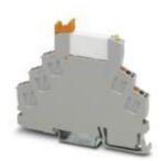
Pre-assembled relay module with push-in connection, consisting of: relay base with ejector and power contact relay. Contact type: 1 PDT. Input voltage: 24 V DC
