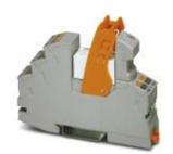
Pre-assembled relay module with push-in connection, consisting of: relay base, power contact relay, plug-in display/suppressor module, and retaining bracket. Contact type: 2 PDTs. Input voltage: 120 V AC
