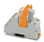
Pre-assembled relay module with push-in connection, consisting of: relay base, power contact relay, plug-in display/suppressor module, and retaining bracket. Contact type: 4 PDTs. Input voltage: 120 V AC
