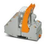
Pre-assembled relay module with push-in connection, consisting of: relay base, power contact relay, plug-in display/suppressor module, and retaining bracket. Contact type: 3 PDTs. Input voltage: 120 V AC
