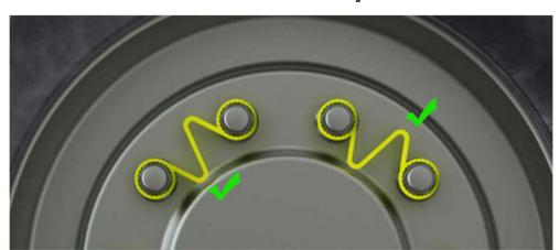
Although still functional, it is not recommended to fit Checklink where a 'd' and 'p' can be seen. Remembered as 'don't put like this ' fitting:
