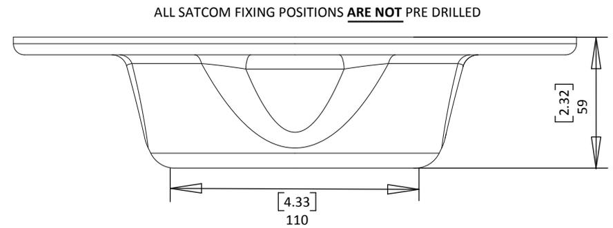
ALL SATCOM FIXING POSITIONS **ARE NOT** PRE DRILLED
