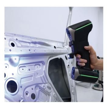
Intelligent edge inspection: It boasts an optional module for intelligent edge inspection. With high-precision gray value measurement, users can inspect closed features precisely and obtain repeatable measurement results.
