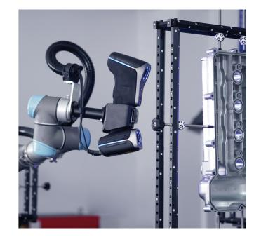
Automated 3D system: It can be paired with Scantech's automated 3D inspection system, enabling effortless deployment and intelligent control to conduct automated batch inspections.
