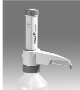
**Variable:** Loosen the volume selector thumb screw by one turn (1), slide the pointer vertically to the desired volume (2) and re-tighten the volume thumb screw (3).
