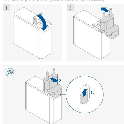
For removing the exchangeable adapter, push the latch upward firstly.
