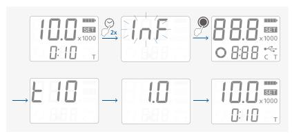
When the device Information setting is active, a self-check screen, the device name, and the software version will appear.
