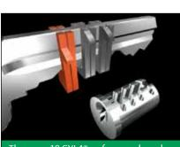
There are 10 CYL4® wafers numbered 0-9, that cover the 10 depths of a C4 key. Six wafers are arranged in pairs to match the first 3 cuts of the customer's key.
