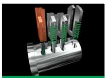
The patented CYL4® cylinder has been designed to retain its wafers when the key is removed. This makes re-keying the CYL4® cylinder quick and easy for retailers and locksmiths alike.
