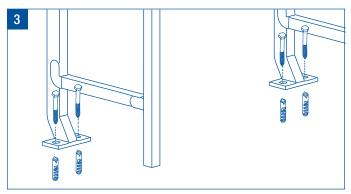
**Fixing**: Drill spot marks with 10mm bit. Screw seat to floor using the Grade 304 Stainless Steel M8 x 75mm hexagon coach screws supplied and 10mm plugs supplied.
