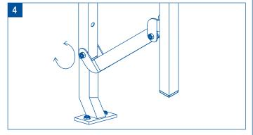
**Checking:** Check seat is firmly secured to the floor and the Tension Grip Hinge screws are appropriate for ease of movement.
