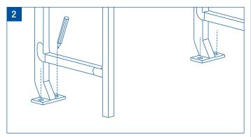
**Positioning:** In the horizontal position, level check and spot mark floor through seat frame mount holes.
