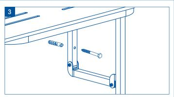
**Fixing:** Drill spot marks with 10mm bit. Plug and screw seat to wall using the 304 Stainless Steel M8 x 75mm hexagon coach screws supplied.
