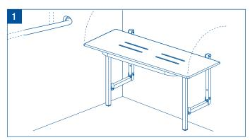
Accessible: Install as per AS 1428.1 Design for Access and Mobility. When in the horizontal position ensure seat does not present a hazard and the grab rail is accessible.
