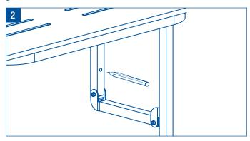
**Positioning:** In the horizontal position, level check and spot mark wall through seat frame mount holes.
