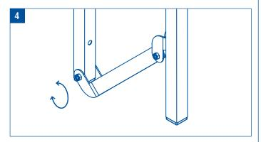
**Checking:** Check seat is firmly secured to wall and the Tension Grip Hinge screws are appropriate for ease of movement.
