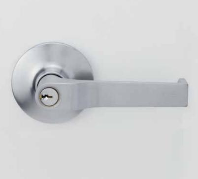
The new AS1428.1 Lockwood compliant leverset features a right angle return of 20mm length and good clearance from the door to prevent fingers slipping off during use. A push button on the interior side lever of the Exterior and Privacy Sets allows a single action egress function. This leverset is designed to enable positive grip and is suitable for door thickness of 35mm to 45mm.
