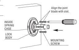
**3C:**Install inside spring cage, Screws should be tightened to its full length.
