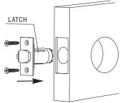
3A: Insert latch unit and fix it with two wood screws.
