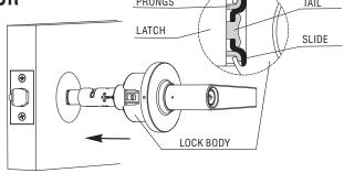
**3B:**Place lock body into position. Make sure that latch prongs engage chassis in housing, and slide engages latch tail.
