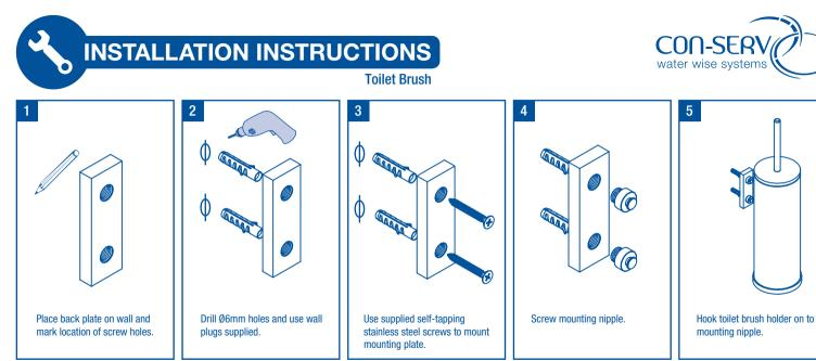
NOTE: If this product is to be installed on a hollow wall, appropriate hollow wall anchors should be used.
