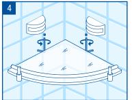
Note: If this product is to be installed on a hollow wall, appropriate hollow wall anchors should be used.
