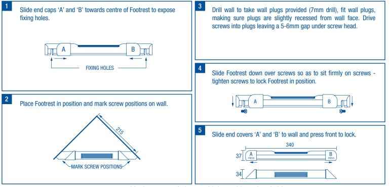
MAX. 70 KILOS LOAD BEARING. STAINLESS STEEL SCREWS ENCLOSED
