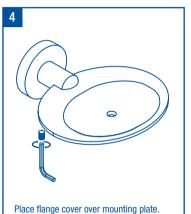
Using the hex key provided, tighten grub
