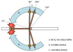
**Note:** Maximum allowable opening angle of 90° for back-check (BC) models
