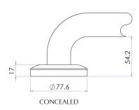
\*50-60mm wall clearance required under most building design codes
