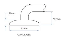
\*50-60mm wall clearance required under most building design codes
