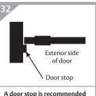
A door stop is recommended on the external door face when using a key locking application.
