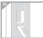
Chisel out strike plate recess. Strike plate must be flush with
