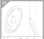
Mark a vertical line down the door jamb, along the edge of the
