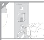
Insert bolt, the drill Ø2mm pilot hole and affix with screws provided.
