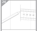
From the verical line on the door jamb, measure and mark half the door thickness. Draw a second line.
