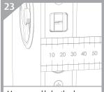
Measure and halve the door thickness.
