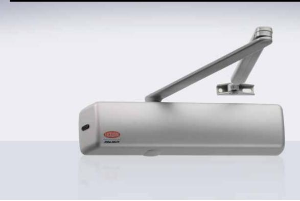
The Lockwood 2657 Heavy Duty Series is suitable for use on internal and external doors and is an ideal solution for extremely heavy doors. Maximum door weight 160kg and door leaf width 1600mm with standard arm installation.
