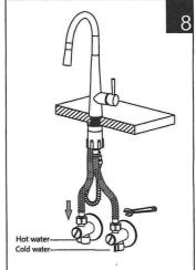
\* Attach two flexible hose to water supply.
