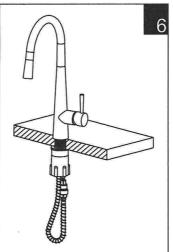
\* Pull out the spray head to check the flexible hose can work properly or not.
