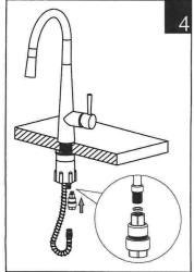
\* Put the paper gasket in the check valve on connector. Then screw with fixing bolt.
