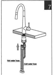
\* Connect hoses to water inlets to Hot & Cold indicators as shown in the figure.
