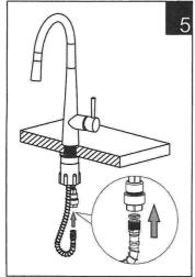
\* Put the rubber washer, Screw the extractable hose with the connector.
