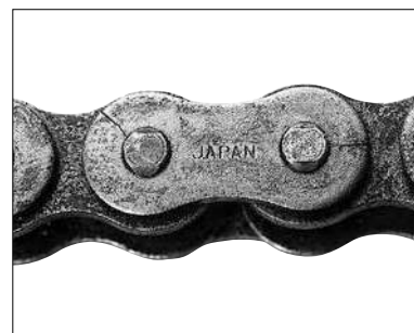
Fig. 35 Hydrogen embrittlement cracking
