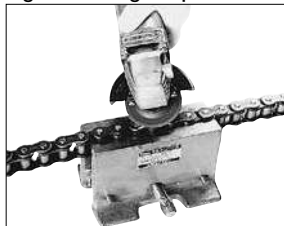
Fig. 2 Grinding the pin ends
