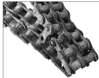
Fig. 34 Corrosion of stainless steel roller chain
