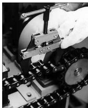
Fig. 9 Connecting between shafts
