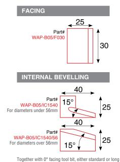
bevelling tool bits are in use depending on pipe diameter. 32mm to 56mm Ø: Long tool bit 56mm to 83mm Ø: Long or short bit 83mm to 114mm Ø: Short bit
