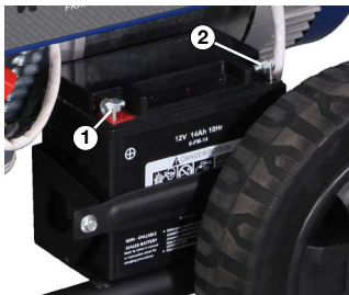
Figure 4 - Battery Connection Order
