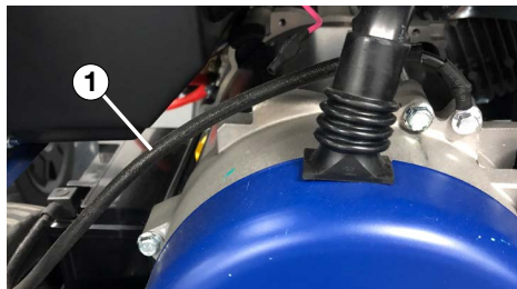
Figure 5 - Locating Negative (-) Cable
