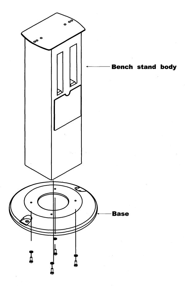
Attach the four (4) bolts and washers through the base and screw into the body of the stand.
