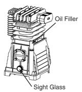
NOTE: The oil must be changed after the first 10 hours of operation then every 50 hours thereafter. Recommended compressor oil:
