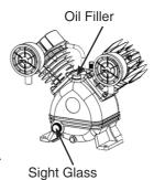
NOTE: The oil must be changed after the first 10 hours of operation then every 50 hours thereafter. Recommended compressor oil:
