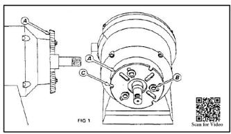
From the right hand end of the grinder, remove wheel cover, wheel, wheel flanges and wheel guard. Fit slotted adaptor plate (A) using either 6mm bolt (3), 5mm Bolt (5) or 4.8mm Bolt (9) from fitting kit. Use appropriate size washers under heads (1 or 12). The outer edge of the adaptor plate is tapered. Face smallest side of taper away from grinder as shown in Fig 1. (A)
