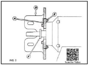
Fit the Main Bracket (D) using bolt (8) through the 3 slots (Fig 1: C) in outer edge of the adaptor plate, with the heads of bolts facing the grinder. With angle face of bracket approximately vertical, tighten 6mm nuts (6) evenly. The adaptor plate should be flush with the main bracket. If the Multitool is to be used in a vertical position simply loosen nuts, tap main bracket (D) to loosen. Swivel to desired position and retighten nuts (6).
