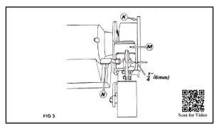
Idler arm Cam plate (M) must now be set 6mm clear of inside edge of the drive pulley (Fig 4. K) Slots are provided under 8mm bolts (Fig 3. J) for this adjustment. Set tracking lever (N) in mid or horizontal position. Fit the belt and release spring loaded contact wheel by lifting the catch (Fig 3. 0)
