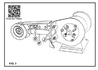
Fit the idler arm (H) using 8mm diameter bolts (2) and washers (7) provided. Fit one of the washers (13) for  $^{1}/_{2}$ " / 12.7mm shafts or (11) for  $^{5}/_{8}$ " / 15.9mm shafts and check that it clears heads of bolts (Fig 1: B). If there is interference, add the required amount of washers to gain acceptable clearance. The drive pulley (Fig 4: K) comes with a 15.9mm bore, there is a 12.7mm steel bush (10) provided for smaller shafts.
