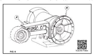
Fit the Drive Pulley (K) by sliding over the shaft of the grinder. Fit tightly against the washer(s) Use 12.7mm (13) or 15.9mm (11) diameter washer (Fig 3. F) under the nut and tighten with a socket spanner.
