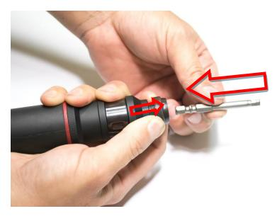
Push the directional switch and plug in the bit to the center.
