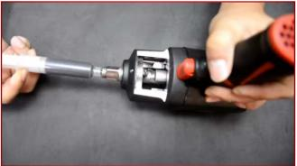
EZ Grease Anvil allows the grease to quickly flow through the anvil and into the casing to coat and lubricate the rotating parts. Benefits of the patented EZ Grease Anvil include:
