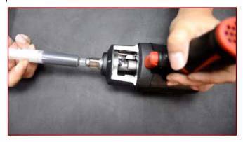
EZ Grease Anvil allows the grease to quickly flow through the anvil and into the casing to coat and lubricate the rotating parts. Benefits of the patented EZ Grease Anvil include:
