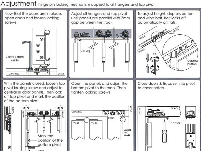
For Top Hung Exterior Folding Door Systems. Non Mortice Aluminium
