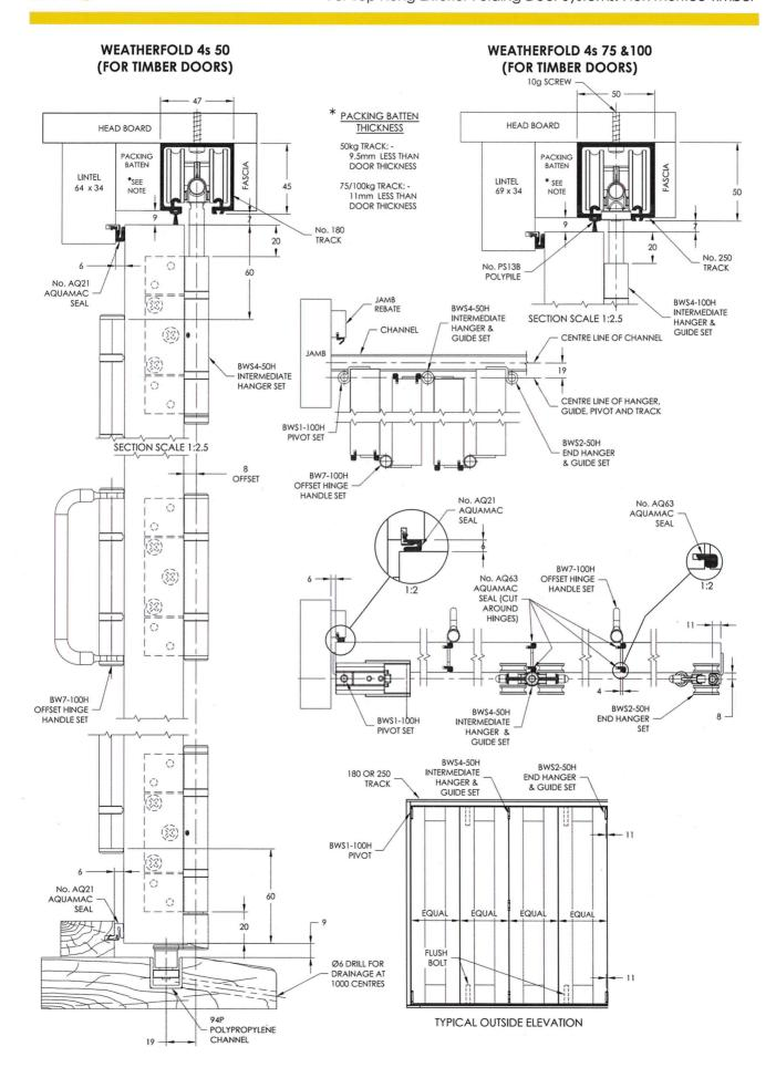
For Top Hung Exterior Folding Door Systems. Mortice Square Timber
