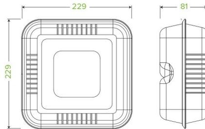
Our plastic-free clamshells are made from rapidly renewable sugarcane pulp, a by-product of the sugar refining industry. Our 9x9x3" white bagasse clamshell containers are an eco-friendly alternative to plastic takeaway containers.
