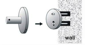
Put the base of bathroom accessory cover on the fixing blocks.
