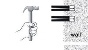
2. Put the expansion plugs into the wall by hammer.
