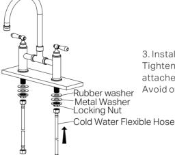
3. Install the rubbers, metal washers and locking nuts.
