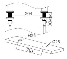
1. Pre-drill or create two holes with diameter of 25mm at the proper location. Please note that the thickness of the surface should be between 3mm-30mm and the distance of two holes is 204mm.
