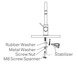
3. Install the rubber and metal washers, if a stabilizer is required, install the stabilizer after positioning the rubber washer. Tighten the screw nut securely by the M8 screw spanner to ensure the mixer is firmly attached to the counter-top. Avoid over tightening to prevent damage to the components.
