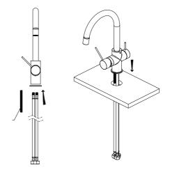
2. Slide the base ring and the O-ring onto the base of the mixer body. Connect the three Flexi hoses and M8 Stud Rod Bolt into the mixer body. Place the mixer body and pass the Flexi hoses through the hole in the counter-top. Ensuring the O-RING sits within the bottom groove of the base plate to prevent water leakage through the cabinet.
