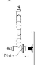
3. Push the plate back to the pot filler body, and screw the pot filler body onto the G1/2 outlet.
