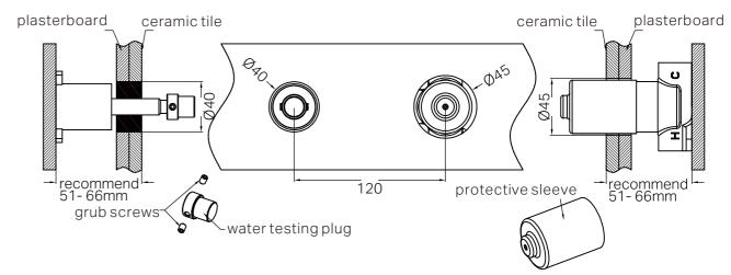
1. Remove protective sleeve, grub screw and water testing plug.
