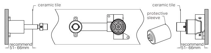
2. Connect cold water hose and hot water hose, take off protective sleeve and conduct water pressure test for leak.
