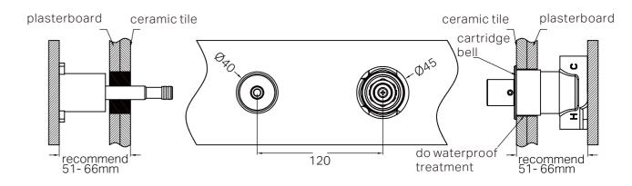
2. Put cartridge bell onto body and do waterproof treatment for the gap between cartridge bell and plasterboard and ceramic tile.
