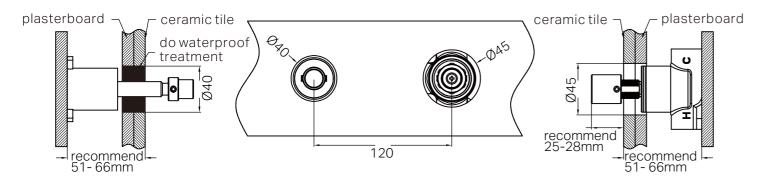
3. Adjust connecting rod and ensure depth is 25-28mm from the front of adaptor to ceramic tile. Drill a  $\phi$  45 and a  $\phi$  40 holes on plasterboard and ceramic tile for the body, according to above picture. Then install plasterboard and do waterproof for the whole plasterboard. Install ceramic tile and do waterproof for the gap between spout outlet and plasterboard and ceramic tile.
