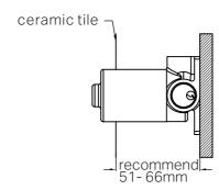
1. Fix body on nogging and ensure installation depth is 51-66mm from nogging to ceramic tile.
