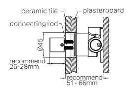
3. Adjust connecting rod and ensure depth is 25-28mm from the front of adaptor to ceramic tile. Drill a  $\phi$  45 hole on plasterboard and ceramic tile for the body, according to above picture. Then install plasterboard and do waterproof for the whole plasterboard. Install ceramic tile.
