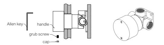
3. Make hand wheel into connecting rod, turn the hand wheel counterclockwise to the end. Then reinstall the hand wheel, make the "C" should be on twelve o'clock direction and "H" on the six o'clock direction, according to above picture. Then tighten grub screw of hand wheel by allen key, put cap into hand wheel.
