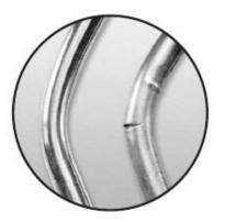
Beside picture shows two ground rods subjected to the same pressure load test.
