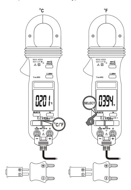
Be sure to insert the banana plug type-K temperature bead probe Bkp60 with correct
